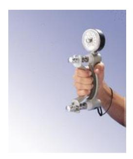
**5.2:** The staff member calibrates the Jamar hand dynamometer at the start of each day by measuring their own grip strength, observing that the needles rise round the dial together and that the red peak-hold needle remains stable and can be read when grip is released. A calibration record is maintained.
