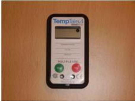
**7.2:** The co-ordinating centre configures the dataloggers to automatically begin recording, this is done before they are sent out to the assessment centre. Therefore the assessment centre does not need to press the start button. A symbol of a sun will be present on the datalogger screen to indicate it is set to automatically begin recording (figure 9).
