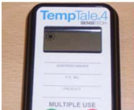
**7.3:** The datalogger is placed on top of the rack within the plastic bag, with this rack at the top of the large transport boxes or mediporter. This will stop the datalogger being inadvertently switched off in transit.
