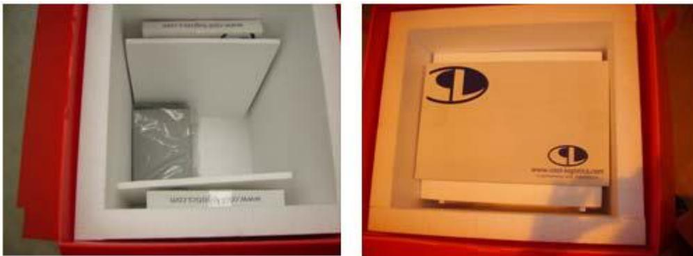
**5.7:** A third spacer is placed on top once the sample racks are all loaded and the third cool pack is placed on top of the spacer (figure 6).
