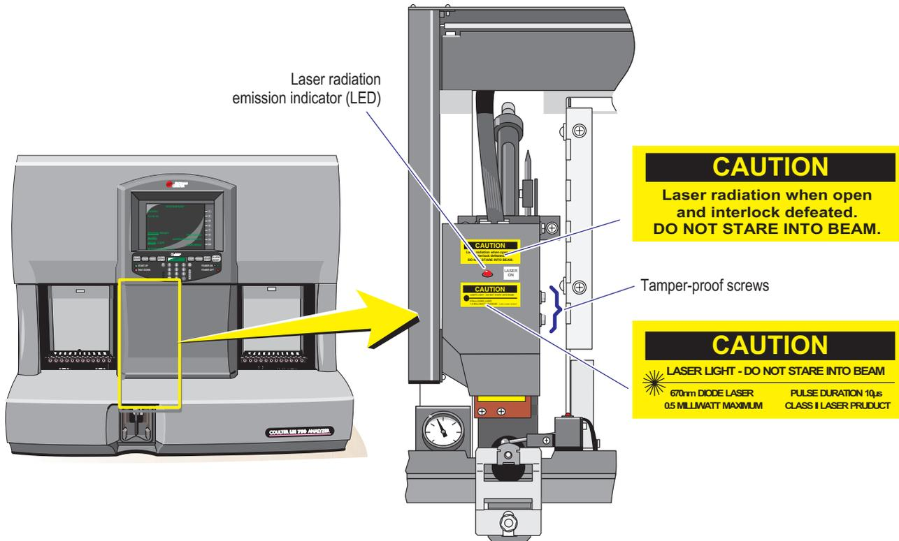
Note: As installed in the Bar-Code Reader Assembly, the laser presents no radiation hazard to users and complies with 21 CFR 1040.
