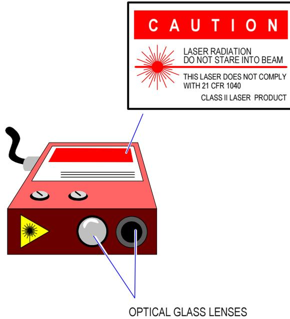
Note: As installed in the Bar-Code Reader Assembly, the laser presents no radiation hazard to users and complies with 21 CFR 1040.
