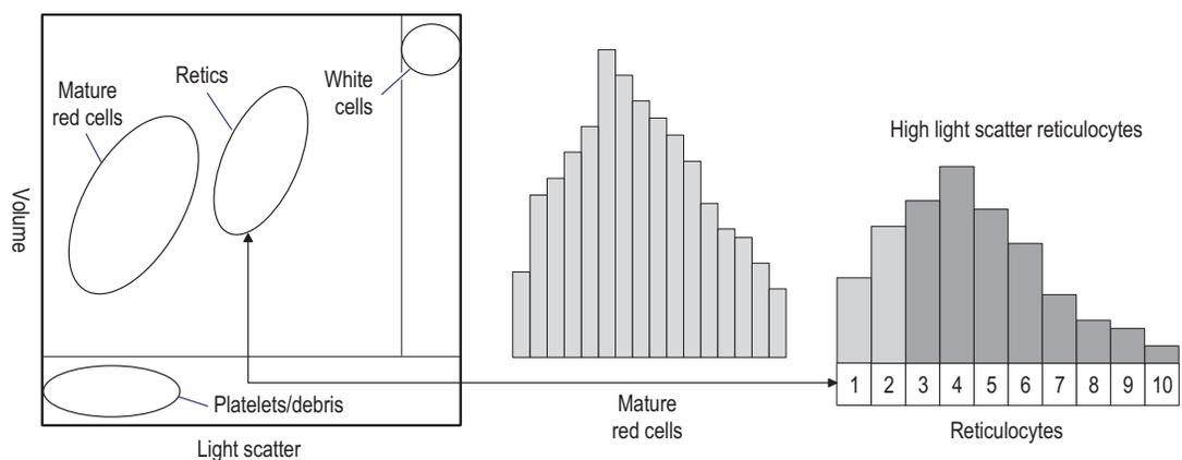
The detected light scatter intensity of the reticulocyte population is divided into the 11 equal regions as shown above. After the reticulocyte population is measured and identified as RET% (regions 0 to 10), the spectrum of light scatter intensity for the identified reticulocyte population is analyzed algorithmically. The RET% is calculated as the ratio of reticulocytes to
