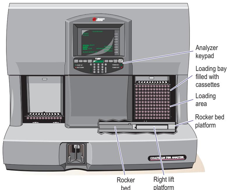
4. The cassette moves onto the rocker bed where it rocks back and forth, mixing the specimens.
