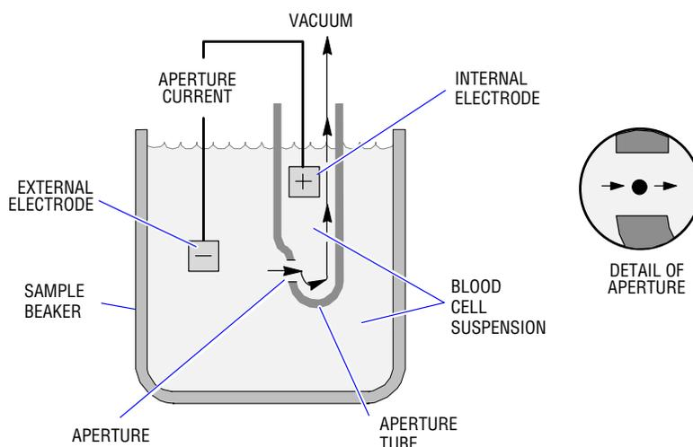
Each cell suspended in a conductive liquid (diluent) acts as an insulator. As each cell goes through the aperture, it momentarily increases the resistance of the electrical path between two submerged electrodes, one located on each side of the aperture. This causes an electrical pulse that can be counted and sized.
