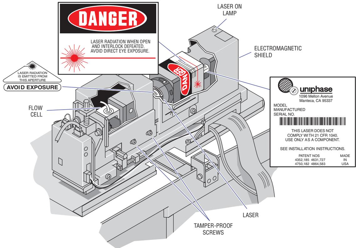
**Note:** As installed in the Triple Transducer Module (TTM) safety fixture, the laser presents no radiation hazard to users and complies with 21 CFR 1040.
