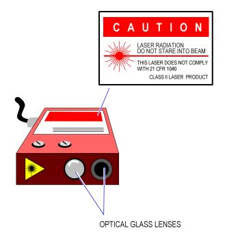
Note: As installed in the Bar-Code Reader Assembly, the laser presents no radiation hazard to users and complies with 21 CFR 1040.
