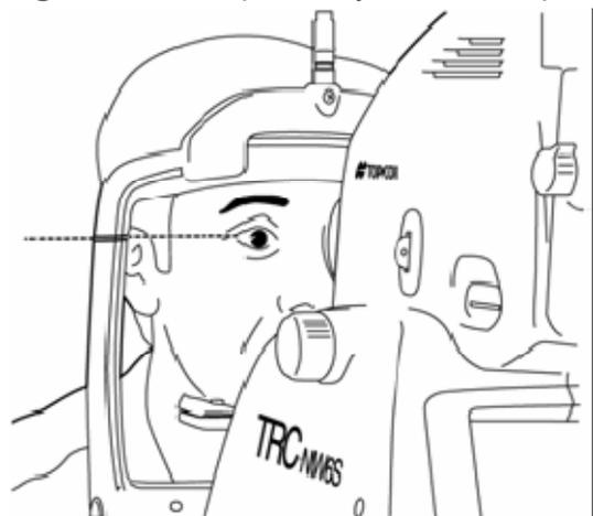
**4.10:** The instrument body is positioned close to the operator and towards the L or R side (according to which eye is being scanned) in order to visualise the eye. It is checked that the TOPCON screen correctly displays the side being scanned (by showing the letter L or R on the display screen).
